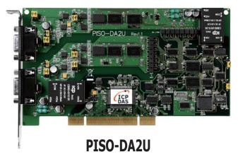
Universal PCI, 2-ch Isolated Analog Output Board
